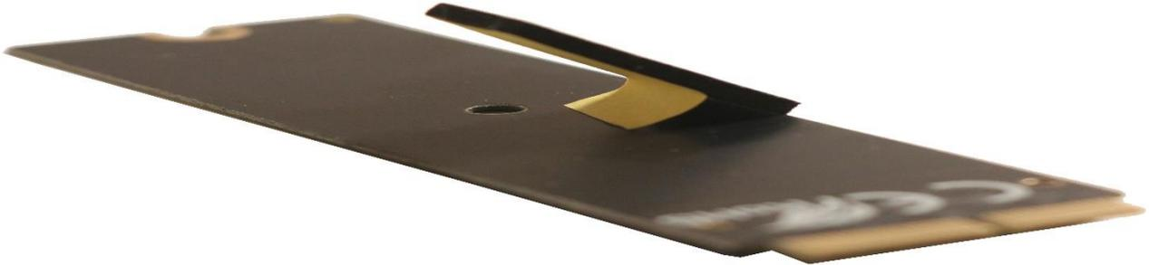
Put Place the NVMe SSD of your choosing into the adapter. The screw cutout should lineup nicely between the two items.
